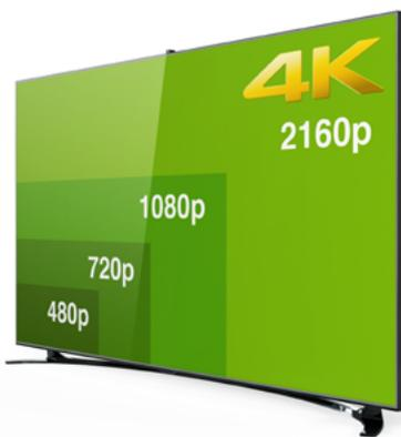
The 4K standard defines 2160 points for vertical resolution, which means an effective picture size four times HD size (1080p). Unless any optimization occurs, preserving the same granular image accuracy from HD would result in a stream 4 times heavier to store and 4 times larger to deliver in 4K.
